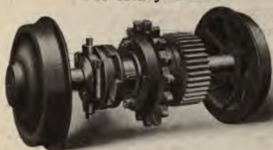
Driving Arrangement for Combination Traction and Rack Operation
